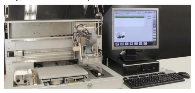
The optional PiXDRO DMC module is available as upgrade for your PiXDRO system. It is completely integrated and can be controlled from the printer's user interface software just like other heads. It can be used with all available cartridges for 1 and 10 pL drop size (DMC-11601, DMC-11610, DMCLCP-11601, DMCLCP-11610).
